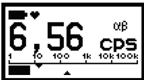
Simultaneous measurement of alpha, beta and gamma radiation
